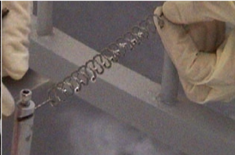
1 of 63 6-inch tungsten filaments being attached to conductive posts.
