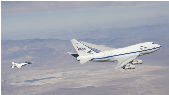
Figure 1. NASA’s SOFIA infrared observatory with chase plane during the first series of test flights to verify the performance of the modified Boeing 747SP. From the NASA Dryden Flight Research Center Photo Collection.
