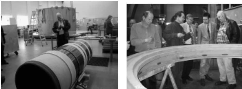
Figure 2. a( left ) SOFIA Nasmyth Tube. b( right ) Forging of the outer support cradle.
