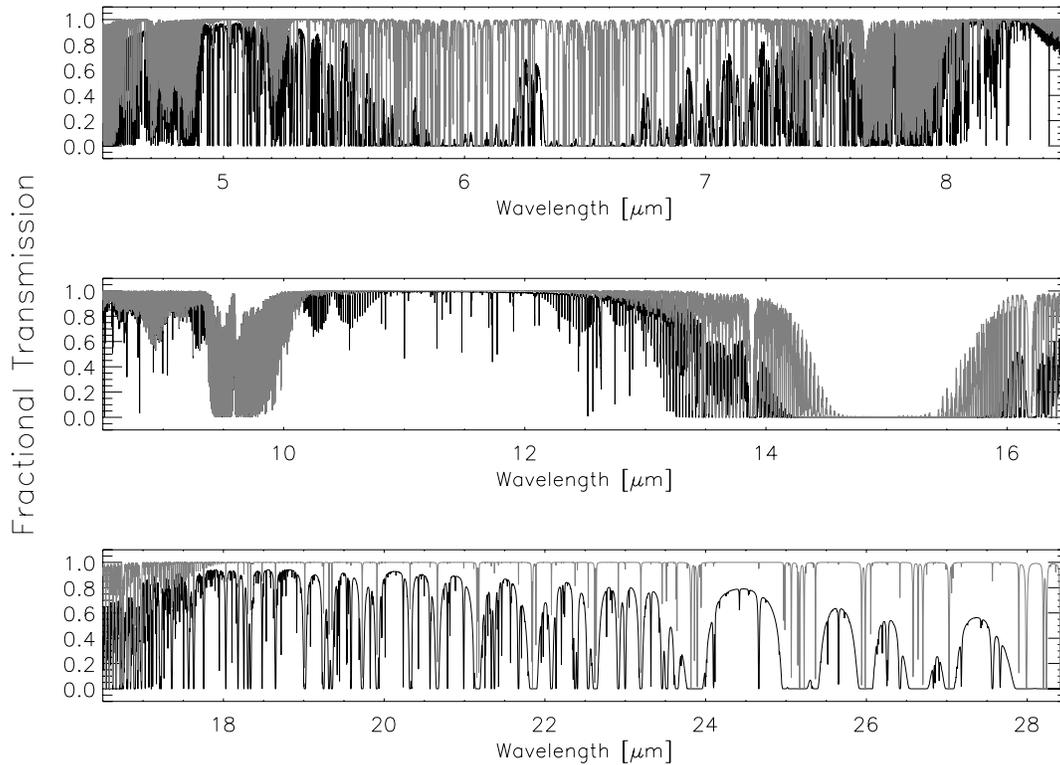
**Figure 3.** A comparison of the atmospheric transmission across the EXES operating range from Mauna Kea (black) and SOFIA (grey). The greatest improvements in the transparency are seen in regions dominated by water vapor such as the 5-7  $\mu\text{m}$  and 20  $\mu\text{m}$  region.
