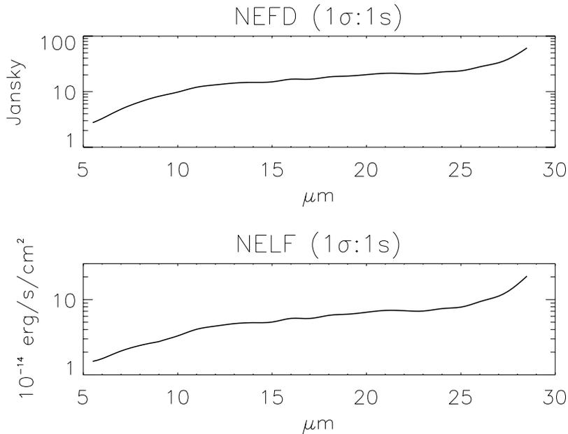
**Figure 2.** Estimated high-resolution sensitivity for EXES on SOFIA as a function of wavelength. The numbers given are  $1\sigma$  for 1 second on-source for a continuum object (top) and an unresolved line (bottom). The estimates assume SOFIA image quality is diffraction-limited for  $\lambda > 15 \mu\text{m}$  and that residual atmospheric transmission is 100%.
