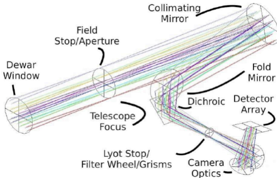
Figure 2. FORCAST optical layout and raytrace of a single camera/channel. Grisms will be located in dual filter wheels located near the Lyot stop.
