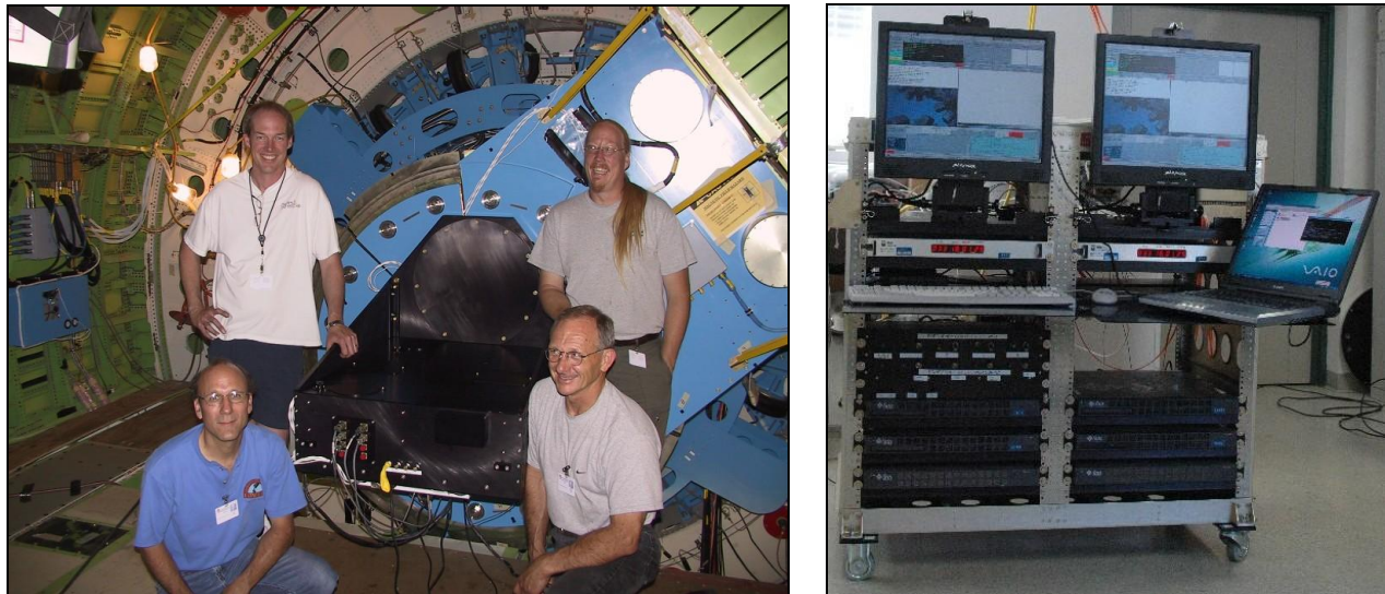
Fig. 1. The instrument, complete except for final cable routing, is shown mounted on the SOFIA telescope during ground operations in 2004 (left) and the completed instrument control rack is shown in the lab (right). The laptop computer on the keyboard tray is not part of the rack configuration, but demonstrates that the tray can carry this load.
